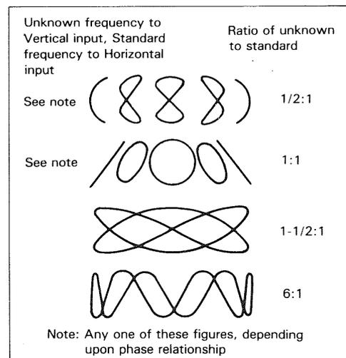
Fig. 44 Lissajous waveforms used for frequency measurement
