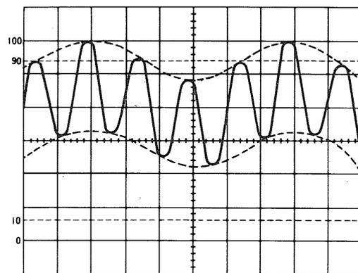
Signal containing undesired component
